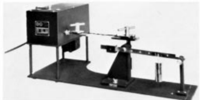
FIG. 1 Device for Preparing Twisted Pair Specimens, Motorized Unit
