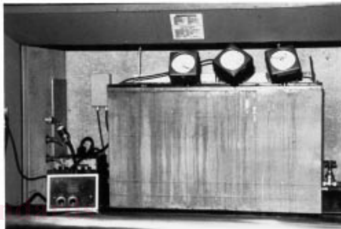
FIG. 1 Rotating Bomb Oxidation Test Apparatus
