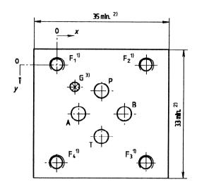
1) The recommended minimum engagement for fixing screws on ferrous mountings is 1,5D, where D is the screw diameter. The recommended full-thread depth shall be 2D+6 mm to aid interchangeability of valves and to reduce the number of fixing screw lengths.
