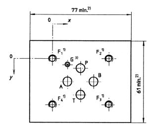
1) The recommended minimum engagement for fixing screws on ferrous mountings is 1.5D, where D is the screw diameter. The recommended full-thread depth shall be 2D+6 mm to aid interchangeability of valves and to reduce the number of fixing screw lengths.
