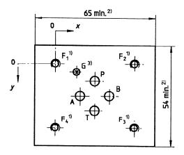
1) The recommended minimum engagement for fixing screws on ferrous mountings is 1,5D, where D is the screw diameter. The recommended full-thread depth shall be 2D+6 mm to aid interchangeability of valves and to reduce the number of fixing screw lengths.
