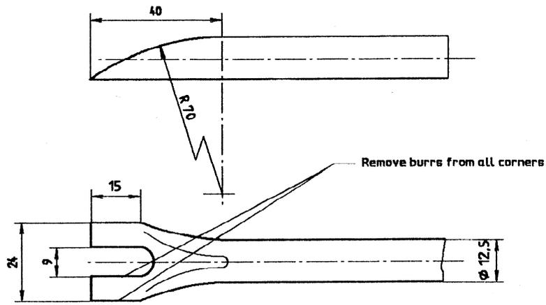
a) Chisels for weld diameter  $\leq 8$  mm
