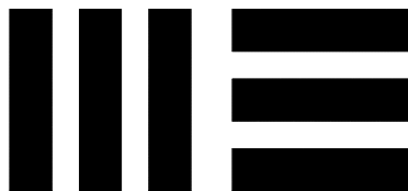
Figure 2 — Test target for checking the resolving power
