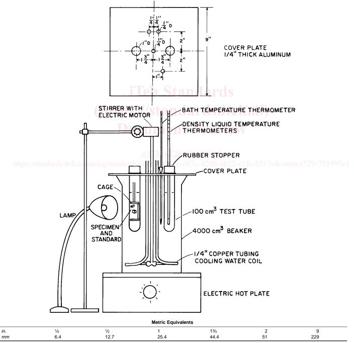
FIG. 1 Single Tube Sink-Float Density Apparatus
