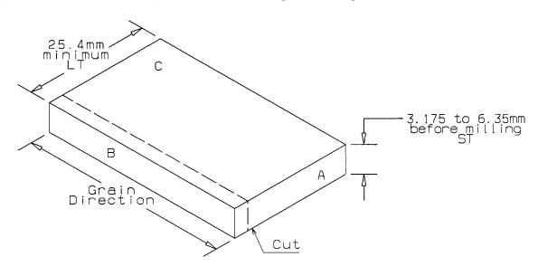
Face A is polished to .812  $\mu m\ R_{a}$  or finer
