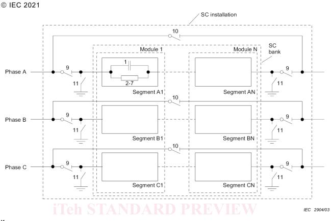
Key1 assembly of capacitor units
