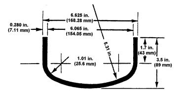
NOTE 1—Caps furnished to ANSI standards unless otherwise specified. Welding caps are formed from steel plate and are ellipsoidal in shape. The minor axis being equal to one half the major axis radii "R" and "r" closely approximate the actual semi-ellipsoidal shape. All dimensions in inches and are in accordance with ANSI B16.9.
