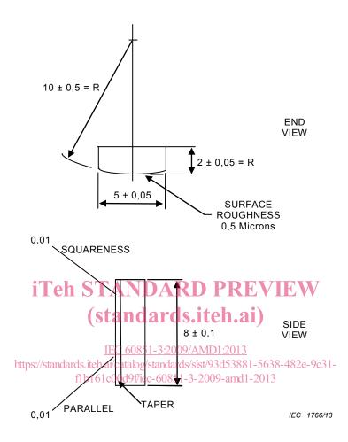
NOTE Dimensions used in the figure are in millimetres.
