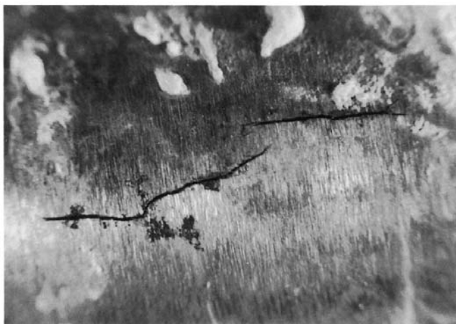
FIG. 2 Typical External Stress Corrosion Cracks (5× Magnification)
