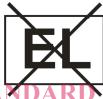
Figure 3 – Lamp not suitable for emergency operation
