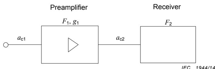
**Figure J.1 – Receiver with preamplifier**
