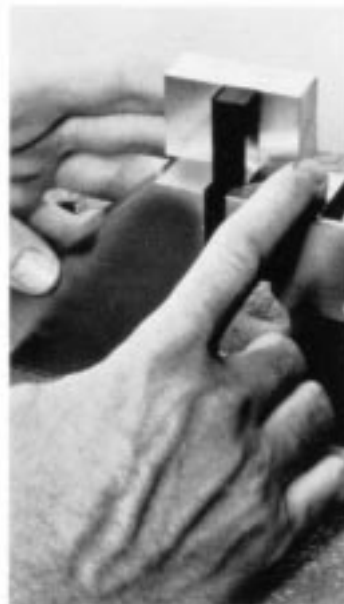
FIG. 4 Jig for Positioning Specimen for Clamping
