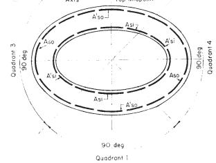
Note 1—The total reinforcement area (A'si) of the inner cage plus the quadrant mat in Quadrants 1 and 2 shall not be less than that specified for the inner cage in Table 1.
