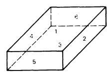
Each angle of intersection shall be identified by the figures designating the two surfaces the junction of which forms this intersection (for example 1-2 identifies the angle of intersection formed by the meeting of the upper surface of the package, No. 1, and the right surface, No. 2).
