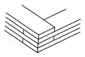
Figure 1. Double-lapped joints
