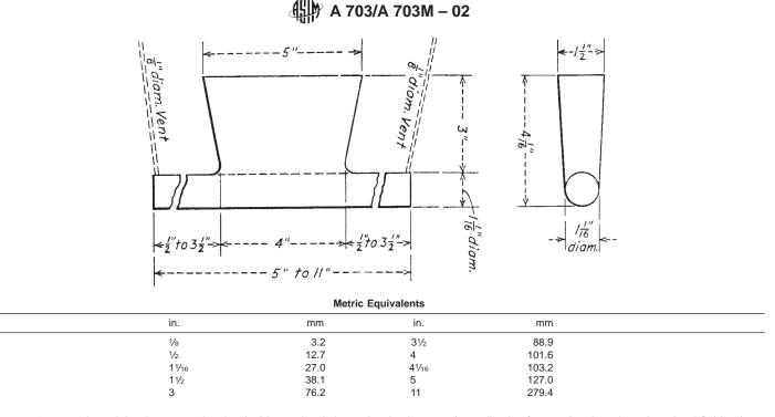
NOTE 1—Pour through head; cover molten head with powdered charcoal, coke dust, etc., immediately after pouring, in order to keep head fluid as long as possible.
