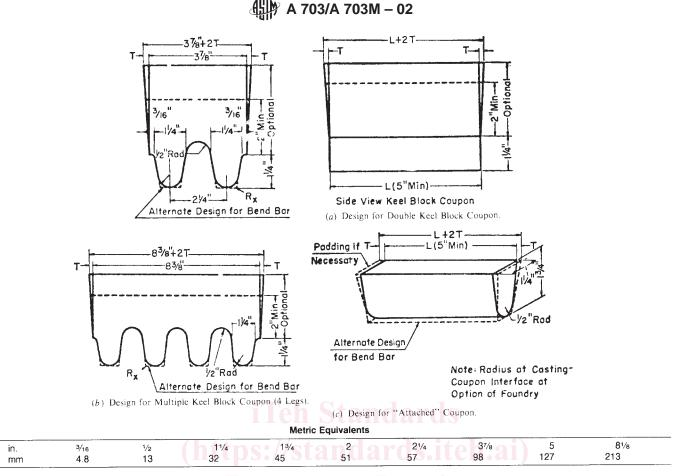
FIG. 2 Test Coupons for Castings (see Table 2 for Details of Design)
