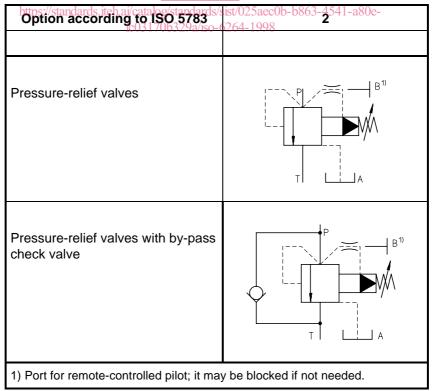
Figure 6 — Pilot-operated pressure-relief valves with main ports of 7,5 mm maximum port diameter (code: 6264-03-04-\*-97)
