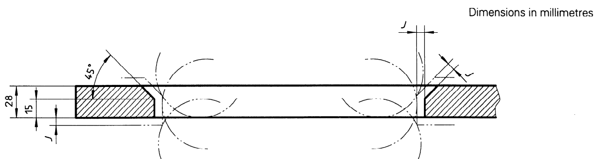
Figure 3 — Minimum clearance between trail wheels and pallet opening
