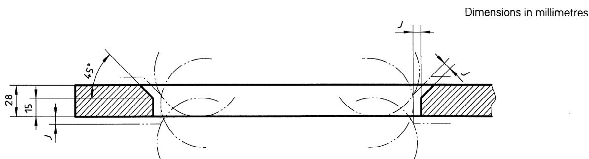
Figure 3 — Minimum clearance between trail wheels and pallet opening
