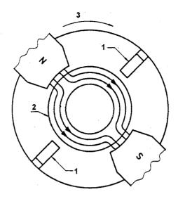
1= magnetic transducers 2= tube 3= rotation of magnets and transducer
