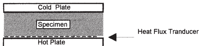
FIG. 1 Apparatus with One Heat Flux Transducer and One Specimen
