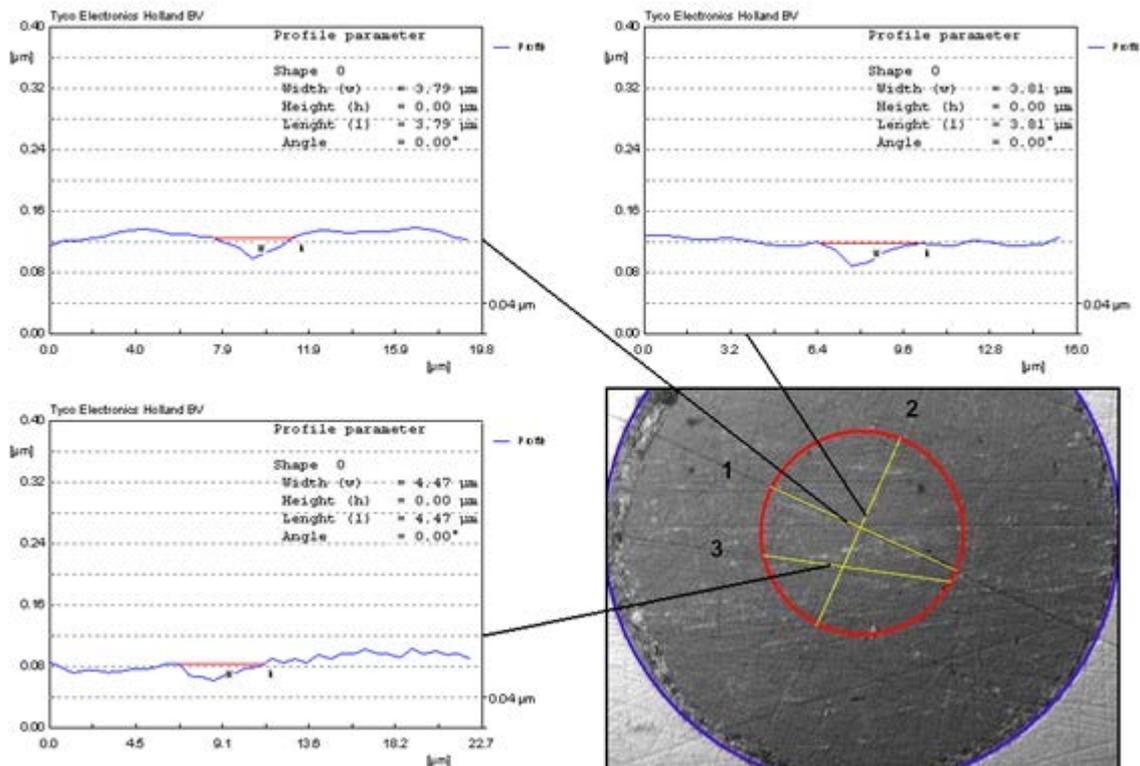
Figure 4 – Examples of characterized endfaces using confocal microscope [7]
