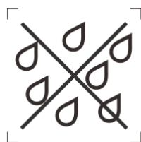
Figure 6 – Lamp not suitable for use under moisture
