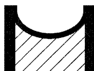
iTeh STANDARD PREVIEW Figure 4 — Profile of the pulley (standards.iteh.ai)
