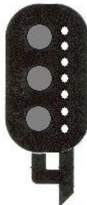
Figure 6 — Example of the colour light signal extinguished with the vertical dot line illuminated
