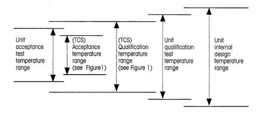
Figure 2 —Temperature definitions for unit thermal design
