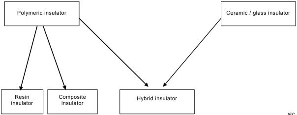
Note 1 to entry: The mechanical functions are mainly characterised by the core, the electrical functions are mainly characterised by the polymeric housing. The housing may cover the core completely or partly. In the latter case the exposed portions of the ceramic core are usually covered by glaze.
