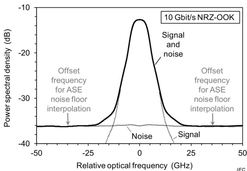
NOTE The signal power is the integral of the power density after subtracting the ASE density. When the spectrum is measured with an optical spectrum analyzer, the resolution bandwidth is often chosen wider than the complete signal, so that the peak of the measurement trace represents this integral.
