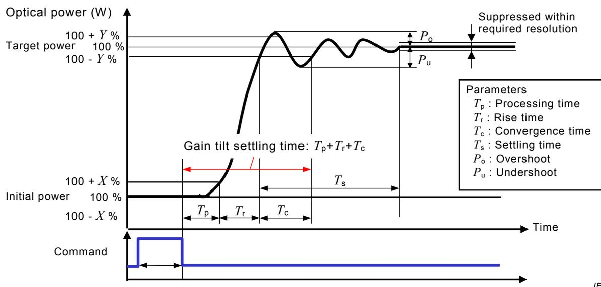
Figure 2 – Response waveforms for digital control DGTEs
