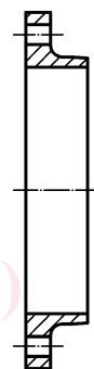
Type 12 Hubbed slip-on flange in copper alloy, for soft soldering, brazing or welding
