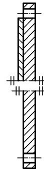
Type 05, 05C 05 Blank flange in copper alloy 05C Blank flange in steel clad with a copper alloy jointing face
