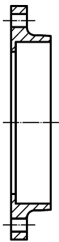
Type 14 Hubbed slip-on flange in copper alloy supplied with tube stops, for soft soldering, brazing or welding
