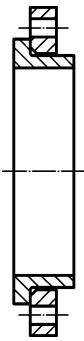
Type 07, 37 Loose plate flange in steel with a slip-on collar (type 37) in copper alloy, for soft soldering, brazing or welding
