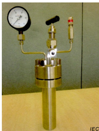
Figure 1 – Autoclave example for ageing test of EIM
