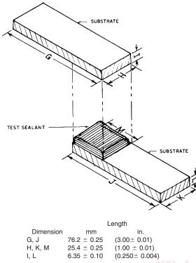
FIG. 1 Assembly of Test Sealant on Substrates
