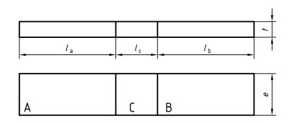
Dimensions in millimetres Test assembly  $l_{a} = l_{b}$ е t  $l_{c}$ 10 Figure 1 30 45 15 iTeh **S**J Reference 3.2.2 10 135 15 30 Figure 2 15 Reference 3.2.3 85 30 10 A/B Run-on / Run-off test piece3690:2000 standards/sist/378b2d56-b3ce-4619-93d7-С Centre test piece. NOTE The centre test piece has the same dimensions in all the three cases.
