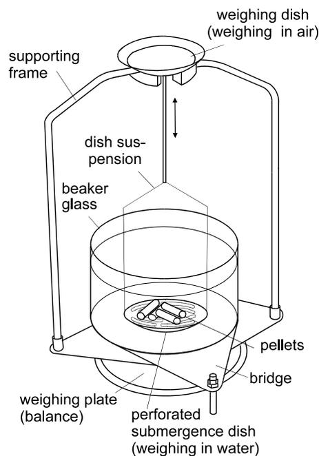
**Figure 1: Buoyancy determination rig on a balance (method for pellets)**
