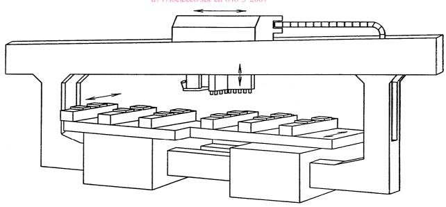
Figure 8 — Example 8 of a portal frame boring machine (moving tables, fixed portal, moving heads)
