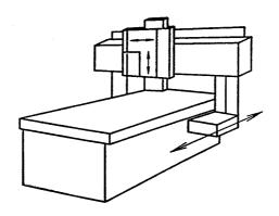
Figure 6 — Example 6 of an overhead router (fixed table, moving portal, moving head)
