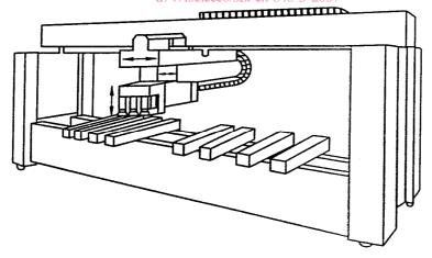
Figure 2 — Example 2 of a portal frame machine (fixed portal, fixed table moving head)
