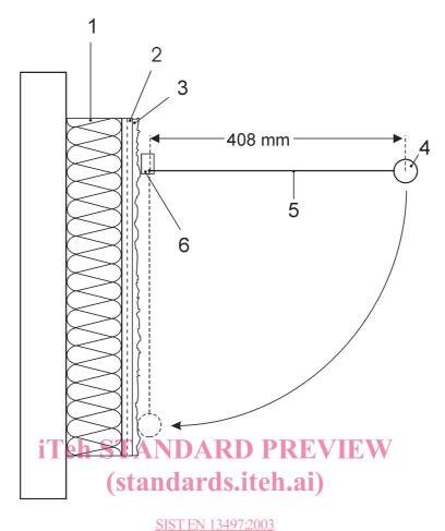
KeySIST EN 13497:20031thermal insulation material sylvatandards.iteh.ai/catalog/standards/sist/sheef/6aff-143f-48db-a9dc-2base coat with reinforcement93918959f2ed/sist-ep-13497-2003<br/>steel wire3finishing material6device for fixing
