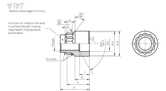
NOTE — Tolerances of form and position shall be in conformity with those specified in ISO 8788. Details of form not stated are at the manufacturer's discretion.
