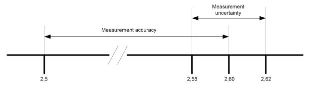
Figure 1 - Measurement accuracy and measurement uncertainty
