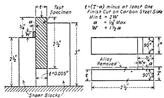
Shear Blocks shall be Bolted Firmly Together against Filler Piece which Provide Space 0.005" Wider than & of Specimen
