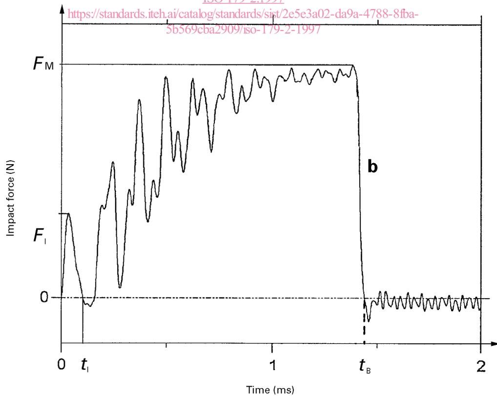
Figure 1 — Typical force-deflection (N and t) and force-time (b) curves
