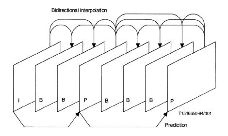
Figure Intro. 1 - Example of temporal picture structure
