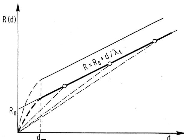
The thickness  $d_{\infty}$  indicates the beginning of the straight portion of the plot of thermal resistance,  $R$ . A reduction of apparatus emissivity shifts the bold line upwards.
