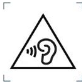
Figure Z1 – Warning label (IEC 60417-6044)
