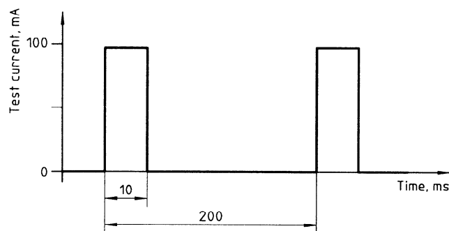
Figure 2 — Example of a test current for environmental simulation
