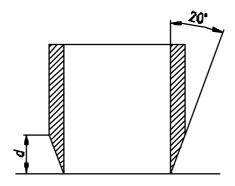
Figure 1 — Design of press knives
