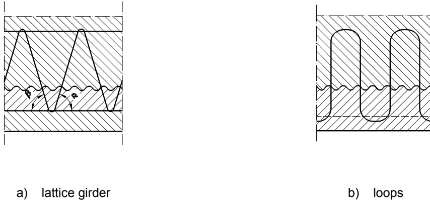
Figure 5 — Examples of shear reinforcements
