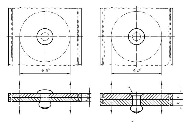
a Countersink angle shall be the nominal angle of the rivet head with the tolerance  $\frac{1}{2^{\circ}}$
